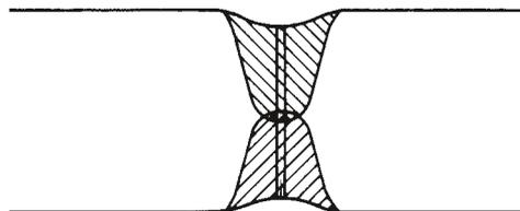
After applying the four diametrically opposed in-depth welding spots, weld the gaps which are still open, covering the tack spots.
