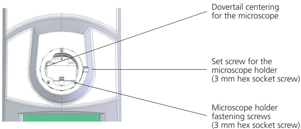
**Fig. 18: Microscope flange (from above)**
