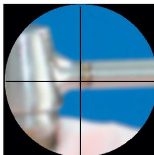
First make sure the reticle is sharp using the adjustment ring,
