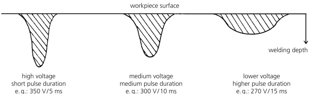
By adjusting the welding parameters, it is possible to join securely solid elements such as lower lingual bars or solid connecting elements, as material thicknesses of up to 4 mm can be welded through by working from both sides. On the other hand, very fine welds (e.g. on implants or precision attachments) can be carried out reliably by reducing the power.
