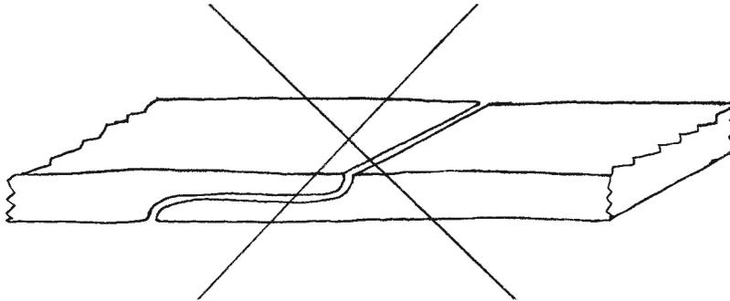
With laser welding, a butt-type contact should always be sought which allows welding from both sides, from above and below.
