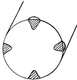
As shown in the diagram, four diametrically opposed welding spots are first applied at low energy. Depending on the application, the welding depth should be between 0.15 and 0.3 mm.
