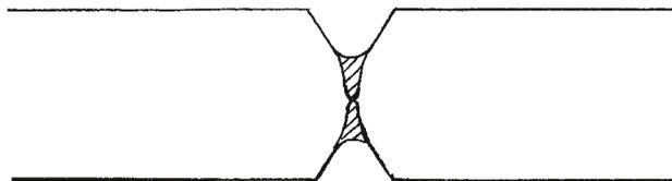
First of all, the centre of the contact surface is welded.
