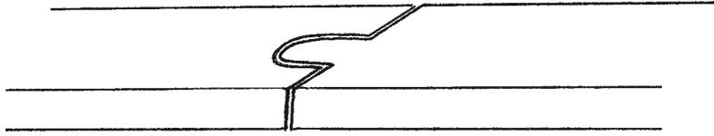
Regardless of how the joint surface is shaped, it must always be possible to weld in the same direction from the opposite side. Only in this way is it possible to equalize any stresses created.
