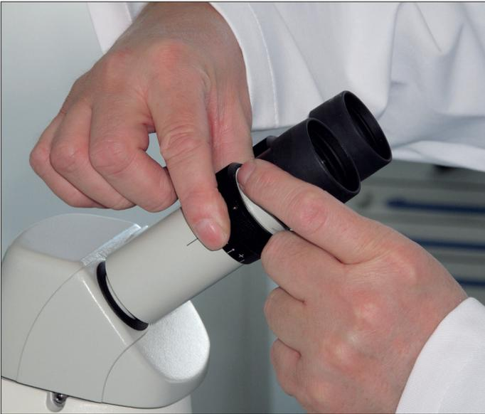
**Fig. 13: Adjust the ocular to the correct individual visual acuity**
