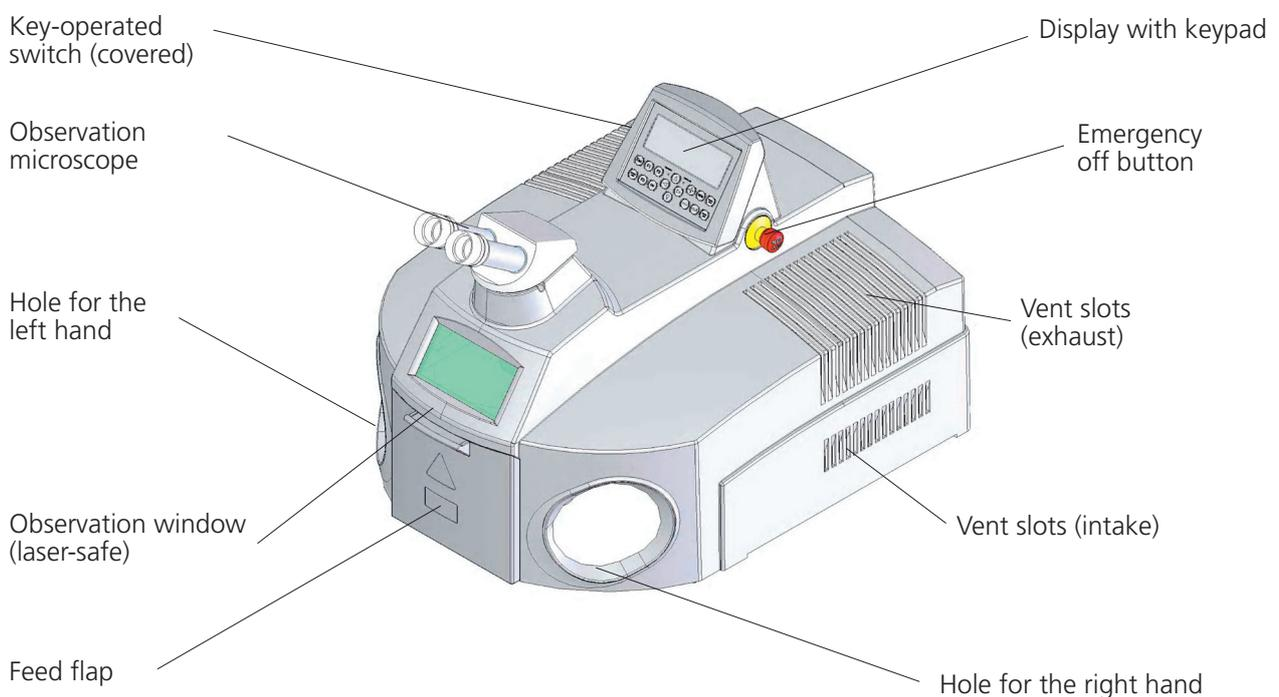
**Fig. 2: Front view of the desktop Compact laser**
