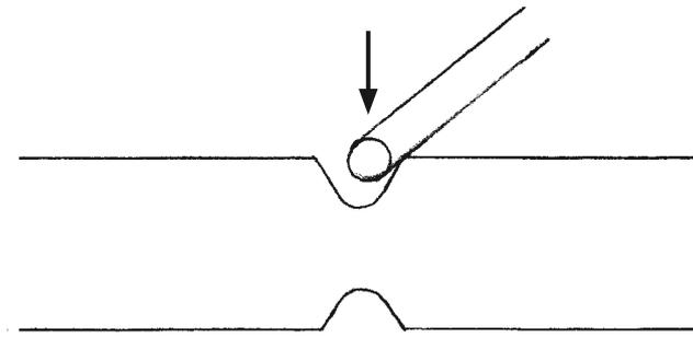
Filler material of the same alloy (wire diameter, 0.35 - 0.5 mm) is applied around the fillet with low welding energy. Sufficient material is added until the overall cross section of the original material is achieved.
