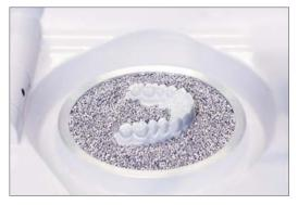
Make sure the edges of the cup are absolutely clean. Heat material by setting the code or recommended heating time according to the instructions. Lock pressure chamber and open once the cooling phase has elapsed.
