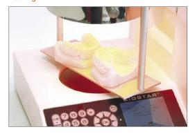
Heat both models for about 3-4 min. under the infrared heater using the heating support (REF 3452, at a distance between occlusal surface and heater of approx. 10 mm). Place both models into the articulator or fixator, position space maintainer and close device slowly. Smooth the lingual area between upper and lower jaw while it is still plastic with moistened fingers.
