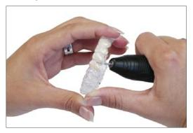
Cut the plate radially and only roughly below the moulded part, remove it carefully from model and finish to exact length.
