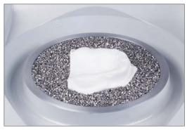
Block out undercuts and single teeth with blocking-out putty. Embed the model to the fold in pellets, so that the model parts which shall be moulded are above the model cup rim. Fill model cup with pellets to the upper rim and make sure the edges of the cup are clean.
