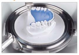
Lock pressure chamber and open after cooling phase has finished. Further finishing is not necessary.
