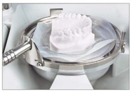
Place the flat trimmed, reduced model on the model platform. When using DURAN® press an ISOFOLAN® foil over the model serving as insulation and and cut the material at the model base with a scalpel. In case of using COPYPLAST® C soak the model in water.
