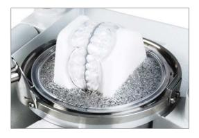
Cut excess BIOPLAST® material with scissors, scalpel or hot knife. Keep distance from the final edges, lay open distal model sides. Take models out of the BIOPLAST® mould and cut surplus material precisely following the definite rim with scissors. Cut the interior shape to its final extension. Expose space holder to insert the air slits and remove it.
