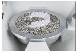
Place model on the platform, in case of high models embed in pellets. Heat the foil by setting the code and recommeded heating times according to the instructions. Lock pressure chamber and open once the cooling phase has elapsed.
