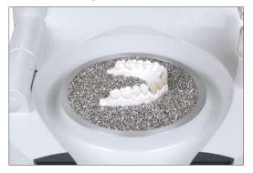
Embed model in pellets, so that the parts of the model to be moulded are above the model cup rim, with the teeth vertically to the foil to be pressed on. Fill model cup rim and make sure the edges of the cup are clean. Heat the material by setting the code or recommended heating time according to the instructions. Make sure the cooling phase is long enough to ensure complete curing of adhesive and primer.
