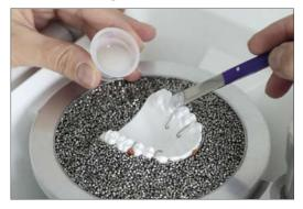
Heat the material by setting the code or recommended heating time according to the instructions. During the last 20-30 sec of the heating time, apply some drops of BIOCRYL® resin to the clasp retentions, close pressure chamber and press heated material over the still liquid resin. BIOCRYL® Resin polymerizes during approx. 20 min. in the pressure chamber and bonds to BIOCRYL® C during this procedure.
