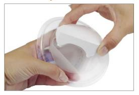
Heat material by setting the code or recommended heating time according to the instructions. Close the pressure chamber and and open once the heating phase has elapsed. The moulded duplicating form should not be trimmed to keep it stable.
