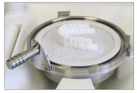
Place model on the model platform or embed it into the pellets in case of high models. Heat material according to the manufacturer's instruction using the programmed code or the recommended heating time. Lock pressure chamber, evacuate and open it once the cooling phase is completed.
