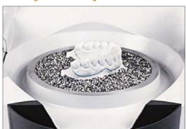
Place upper or lower arch on the model platform resp. embed complete upper or lower model in the pellets and fill model cup up to the upper rim.
