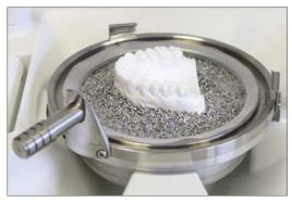
Place the reduced model with flat trimmed model base on the model platform. For insulation, press ISOFOLAN® foil over the model and cut off at the model base using a scalpel.
