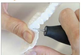
Lift material carefully and cut it to exact length.
