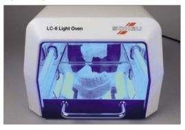
Remove the model with the splint from the articulator and place it centrally in the light curing device. Then cure the material 2 times for 10 minutes each. **Note:** If you intent to cure several splints one after the other, short cool-down phases are recommended. During these cooling phases the drawer of the LC-6 Light Oven should be left wide open.
