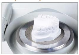
Trim the base of the model flat and soak model shortly in water. Place the plaster model on the platform.
