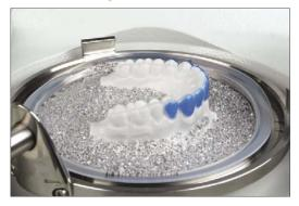
Place dental arcade model on the platform resp. embed complete model in pellets and fill cup up to the upper rim. Pressurize BIOPLAST® bleach or COPYPLAST® depending on the desired stability and model size.
