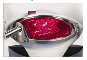
One side of the BRUX CHECKER $^{\otimes}$  foil is colour coated. By scratching the foil margin you can verify the correct fixing of the foil. Heat the foil according to the recommended heating time. Close pressure chamber and open once the cooling phase has elapsed.
