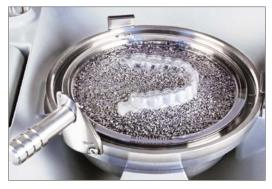
Embed the situation model with brackets in BIOPLAST® segments (refer to picture) and press an ISOFOLAN® foil over it. Heat foil by setting the code or recommended heating time according to the instructions. Lock pressure chamber and open once the cooling phase has elapsed.
